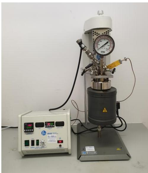
Figure 2. Stirred batch reactor
