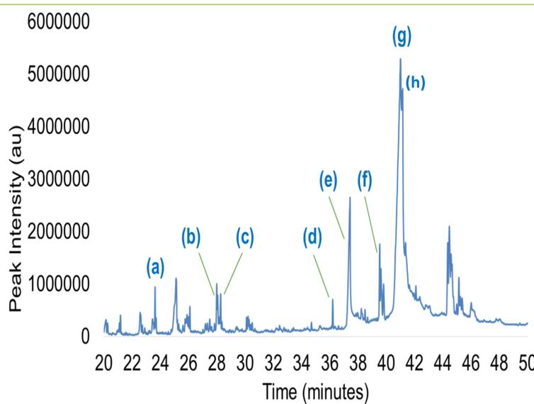
Figure 3. GC-MS Analysis of Liquids from *Jatropha* Oil Pyrolysis at 450 °C
