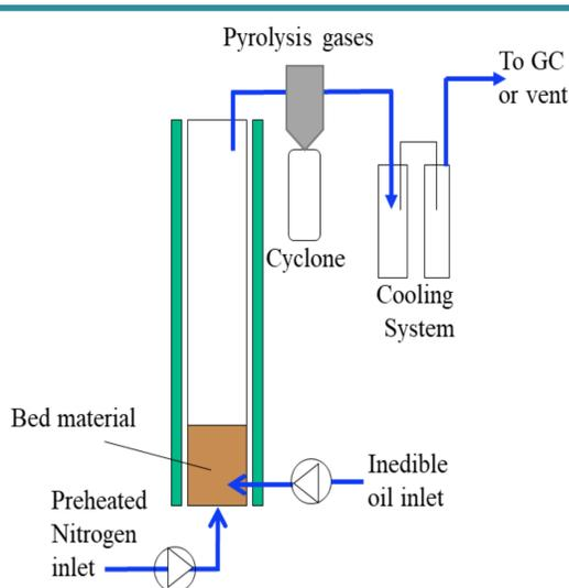
Figure 1. Schematic of Fluidised Bed Fast Pyrolysis Reactor
