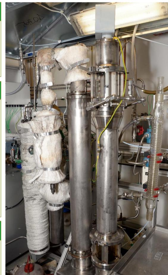
Figure 1. 1 kg h<sup>-1</sup> continuous bubbling fluidised bed reactor including product collection.
