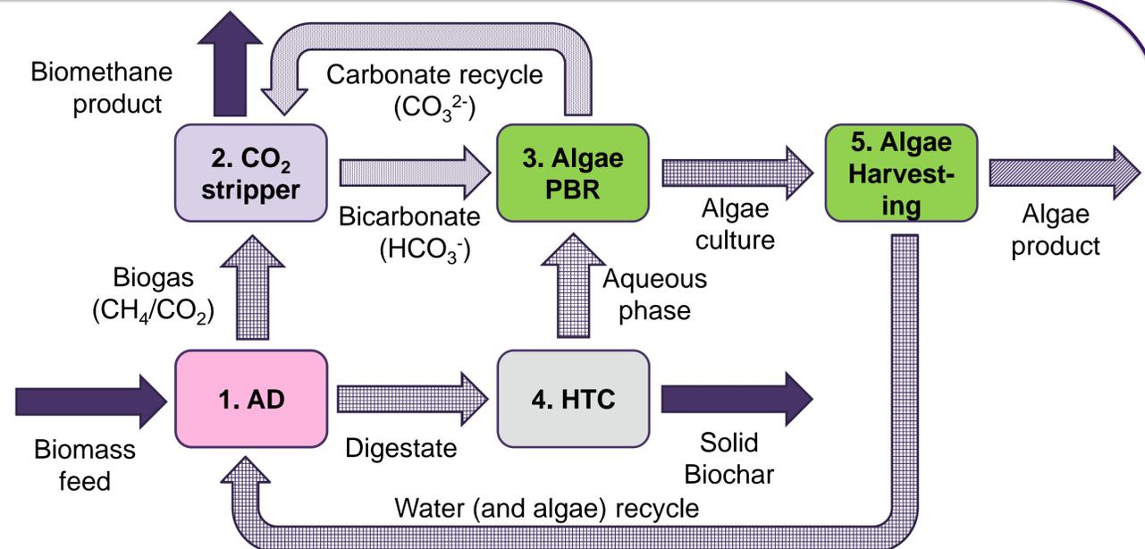
Figure 1. Schematic of integrated process for microalgae-based biomethane purification and carbon sequestration
