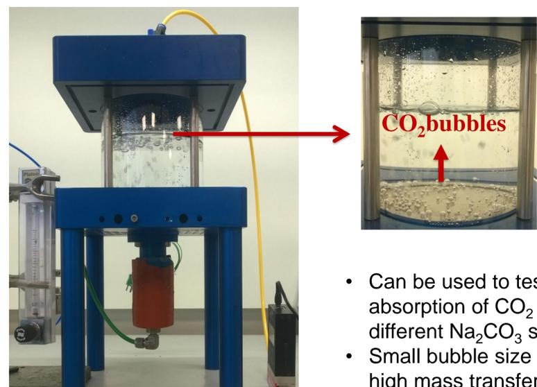
Figure 3. CO<sub>2</sub>-Stripper system
